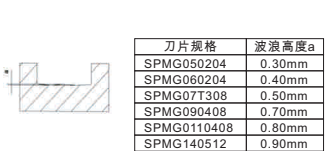
盲孔底面尺寸说明 blind substrate dimension instruction
